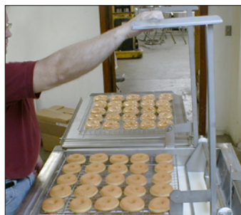
EZLift Mechanism – Tilting to refill applicator
