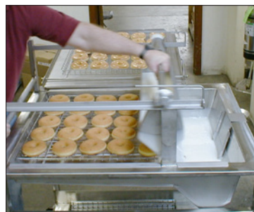
EZLift Mechanism – Glaze Applicator on rails
