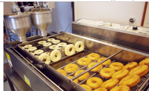
Mark VI Deep with Dual Automatic depositors (for Ring donuts only)
